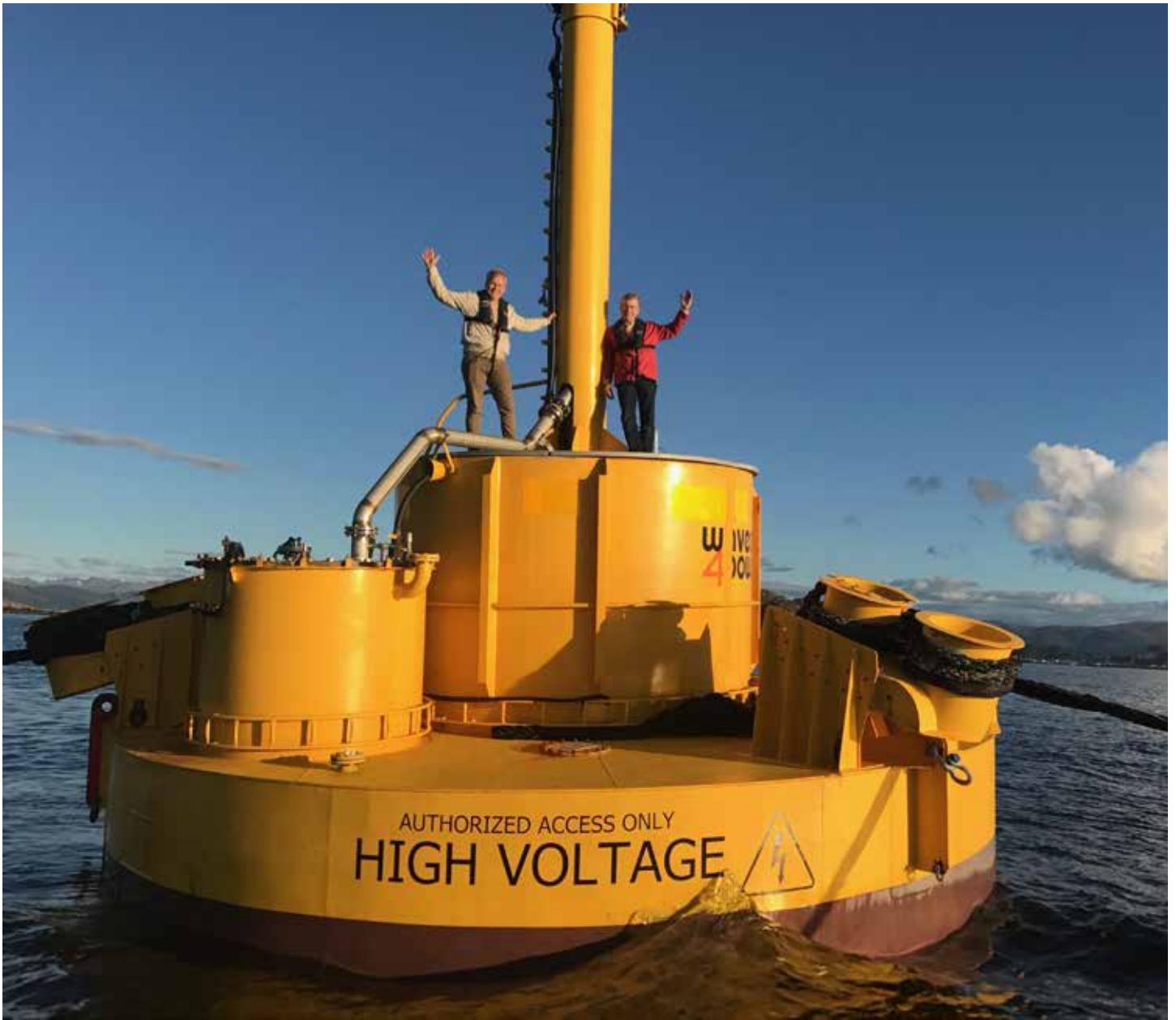
Wave energy project: Over the last few years, Jotun (together with other partners) has supported Waves4Power, a Swedish-based clean energy company. In May 2017, Waves4Power celebrated the successful installation of a buoy, equipped with a wave energy converter, off the island of Runde, Norway. The grid-connected unit is capable of supplying 10-15 normal households with clean power for a year.
