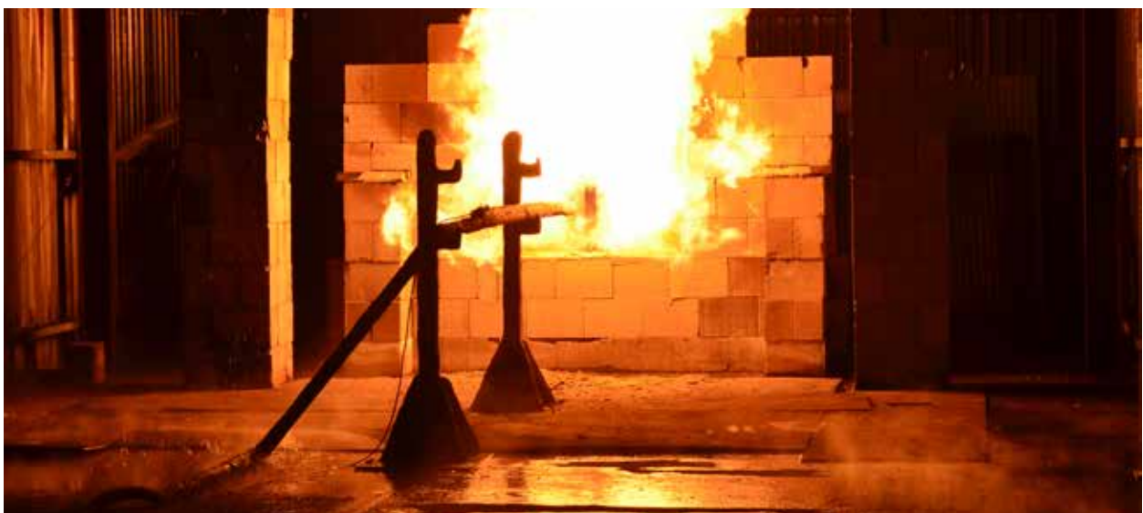
Jotun intumescent Passive Fire Protection test furnace, Dubai U.A.E.
